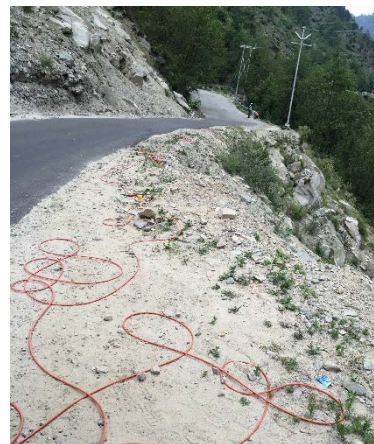
Fig. 5. Seismic refraction test in progress
